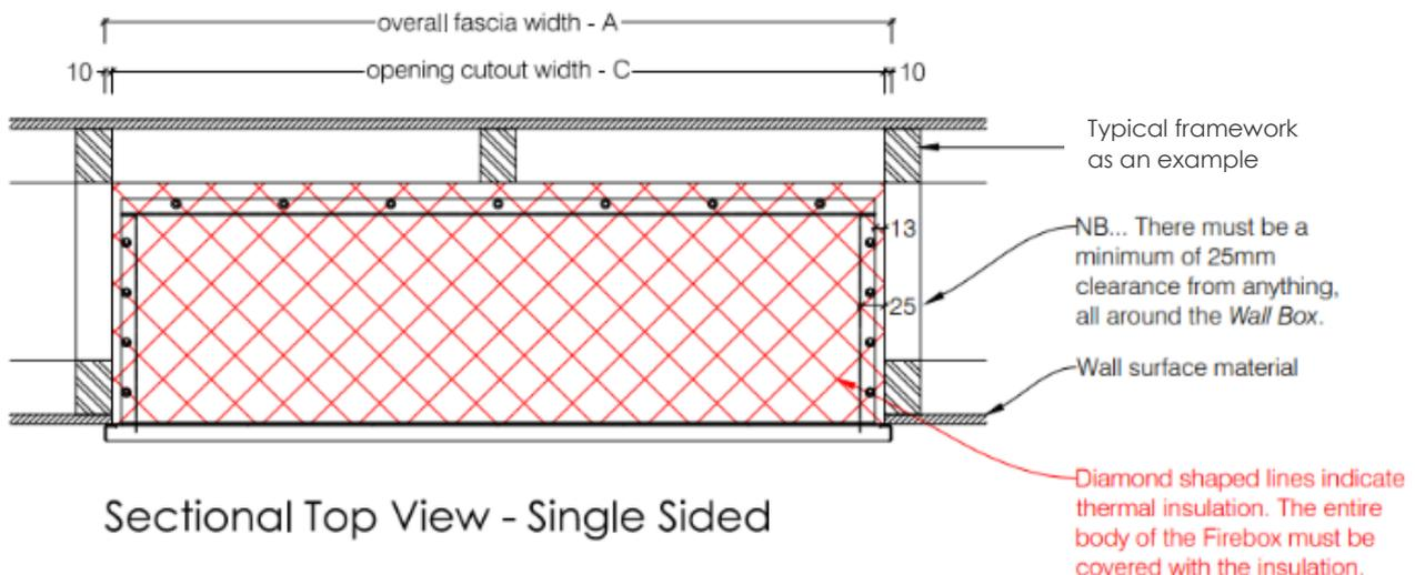
Note: The drawings above are an example of a typical installation using framework and covering the Firebox body with insulation. All installations must comply with the relevant building regulations and restrictions of the country where the installation is to take place.
