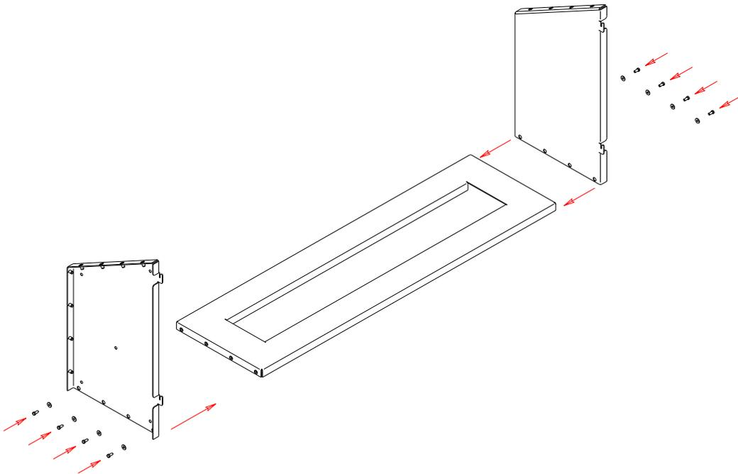
**Place the base plate flat and fix the side plates to the base plate with the fasteners and washers provided. Do not tighten the fasteners completely. Hand fasten only as you might need to make a positioning and adjustments when the other plates are attached. Make sure the base plate front lip (without holes) is on the same side as the highest point of the side plates.**
