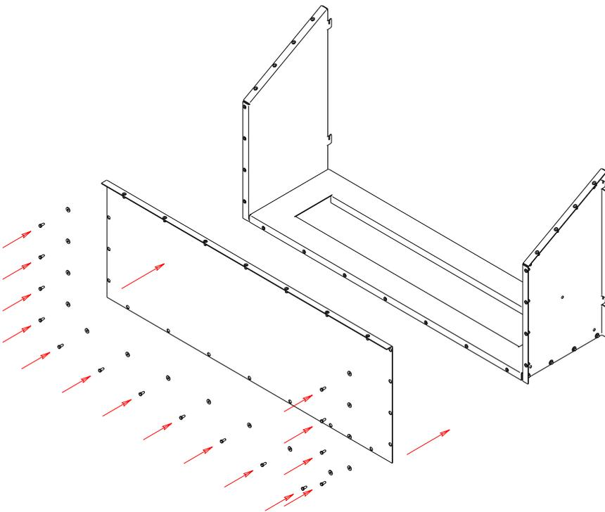
**Next fasten the back plate to the base and side plates. Only hand tighten to allow for positioning and adjustments.**
