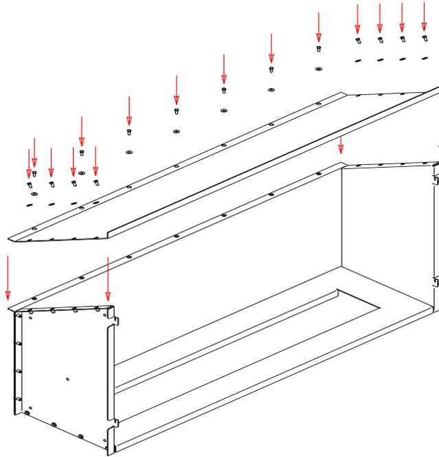
Lastly fasten the top plate to the back and side plates. Make sure all the plates fit together and that there are no gaps visible between the plates. Fasten all the screws tightly. Your firebox is now ready to be installed.
